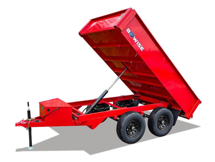
GVWR9,990#PAYLOAD CAPACITY8,030#DECK/BED WIDTH72"HYDRAULICS TYPESingle Acting Hydraulic PumpLENGTH10'CARGO CAPACITY3.3 CU YDSDUMP ANGLE42°COUPLER TYPE2 5/16" A Frame Coupler
